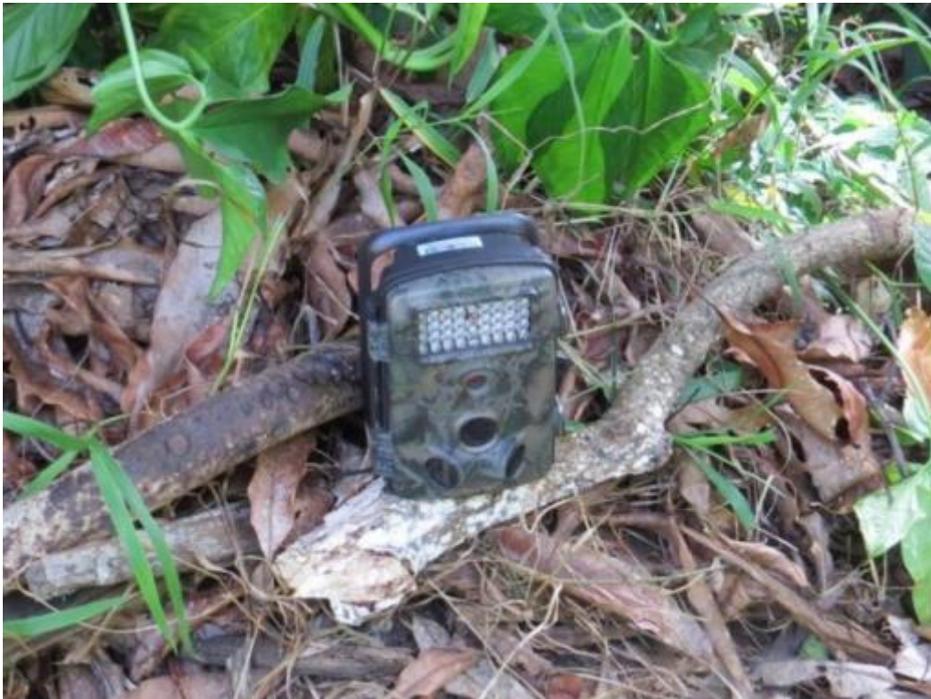
Plate 2(a,b) – General view of Site 1 (Adam’s Ground). The trail camera was placed off the road just to the right of this photograph. It captured images within an angle of about 40° and at night to a distance of about 10 meters. Daytime pictures are in full color, nighttime pictures are black and white.
